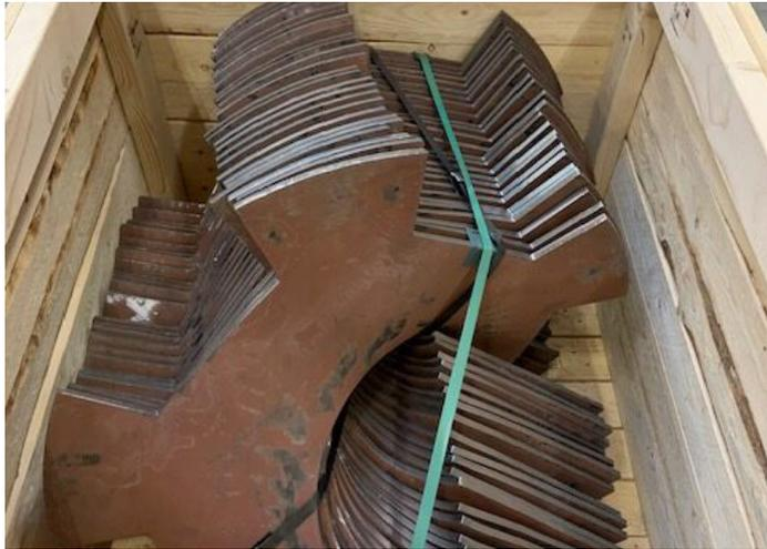
The screw flights have been crafted from Hardox 450 and stainless steel 1.4301/AISI-304 and made with cut offs on the outer diameter. This requires a special design, showcasing our ability to tackle any winding challenge — even when the client is located on the opposite side of the globe.
