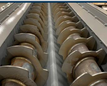
We have delivered a true workhorse for the transport of plastic waste for use in the further processes of one of our customers. The solution consists of two 7,000 mm long rotors (Ø400) mounted in a steel housing. It is painted in the customer-specific RAL color. The auger flights are designed to pack down the transported material, thus making it more uniform for further processing.
