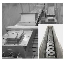
Moistened potato starch is often used in the production of vodka, and correct transportation within its factory facilities is a necessity. BEMA has provided the perfect solution by producing two shaftless transportation screws. Shaftless screws was chosen because humidified starch can be sticky, addressing the importance of being able to transport these materials without sticky coagulation or clogging.
