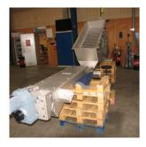
Screw coneyor for ash transport with built in water tank - 24371
