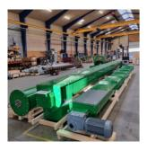
33962 - Screw conveyors for transport of wood chips, including on site montage after shipment
