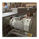
18971 Screw conveyor for drill cuttings
