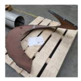
Cylindrical screw flight with cutouts - 34926
