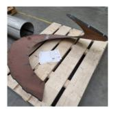
Cylindrical screw flight with cutouts - 34926
