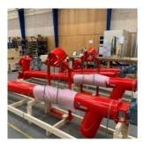
34260 - Screw conveyors in Ø240 ZBEMA and Ø191 for transport of manure
