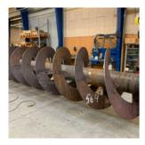
Screw rotor with ribbon flights Ø1520 - 31538
