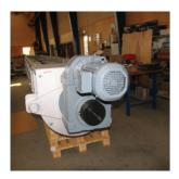
18582 Screw conveyor for high temp ash
